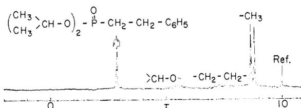
Fig. 9.—Di-2-propyl 2-phenylethylphosphonate (10 vol. % in  $\text{CCl}_4$ ).
